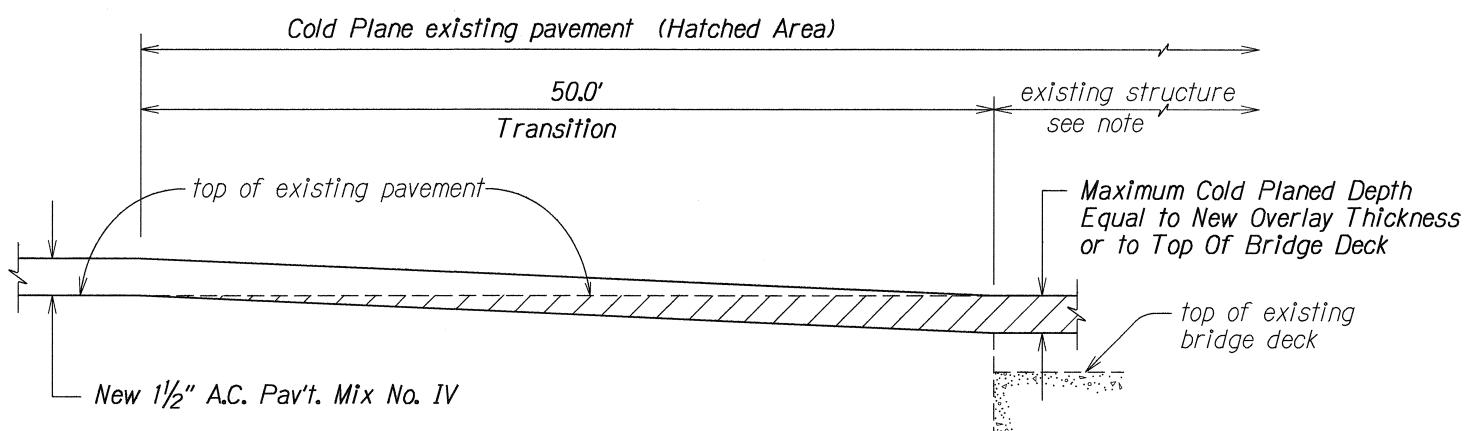
Note: In cold planing the pavement over the structure, the Contractor shall exercise care not to damage any portion of the structure, especially the slab, joints, drainage pipes or reinforcement. Any damage to the structure during the cold planing operations shall be repaired by the Contractor at his expense. Repair work shall be directed by the Engineer. The Contractor shall verify the thickness of the pavement by taking several measurements throughout the structure.
