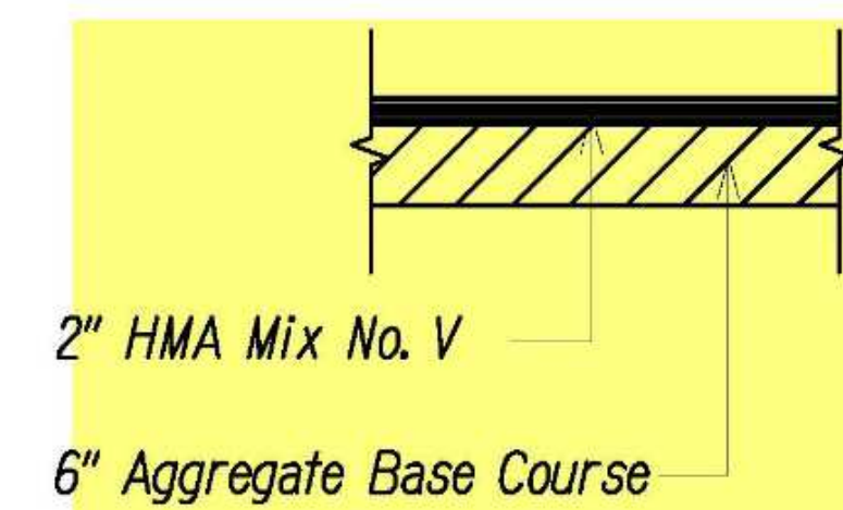
A.C. PAVEMENT DETAIL Scale: 3/4"=1'
