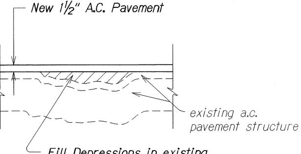
Fill Depressions in existing A.C. Pavement with leveling course of A.C. Pavement Mix No. V
