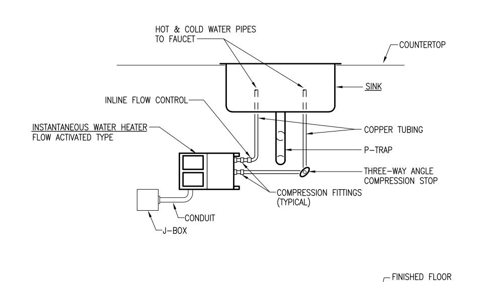
TYPICAL INSTANTANEOUS WATER HEATER DETAIL Р3 NOT TO SCALE
