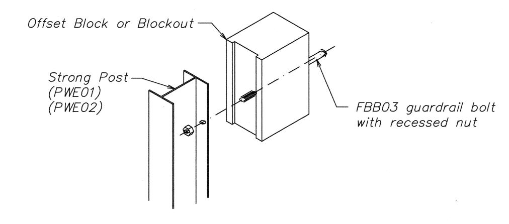
Exploded View (Rail, washer and reflector not shown)
