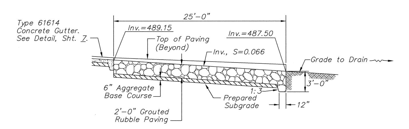
NOTE: Excavation and Backfill, and Aggregate Base shall not be paid for separately, but shall be considered incidental to Item No. 612.0100-Grouted Rubble Paving.
