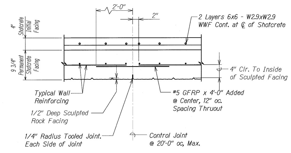
TYPICAL CONTROL JOINTS AT SHOTCRETE WALL Scale: 1 1/2" = 1'-0"
