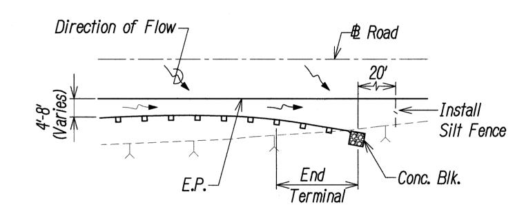
TYPICAL SILT FENCE FOR ANCHOR BLOCK INSTALLATION Not to Scale
