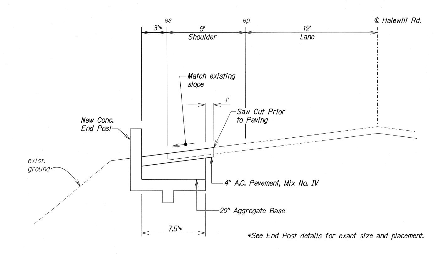
ENDPOST PAVEMENT REPAIR SECTION Not to Scale
