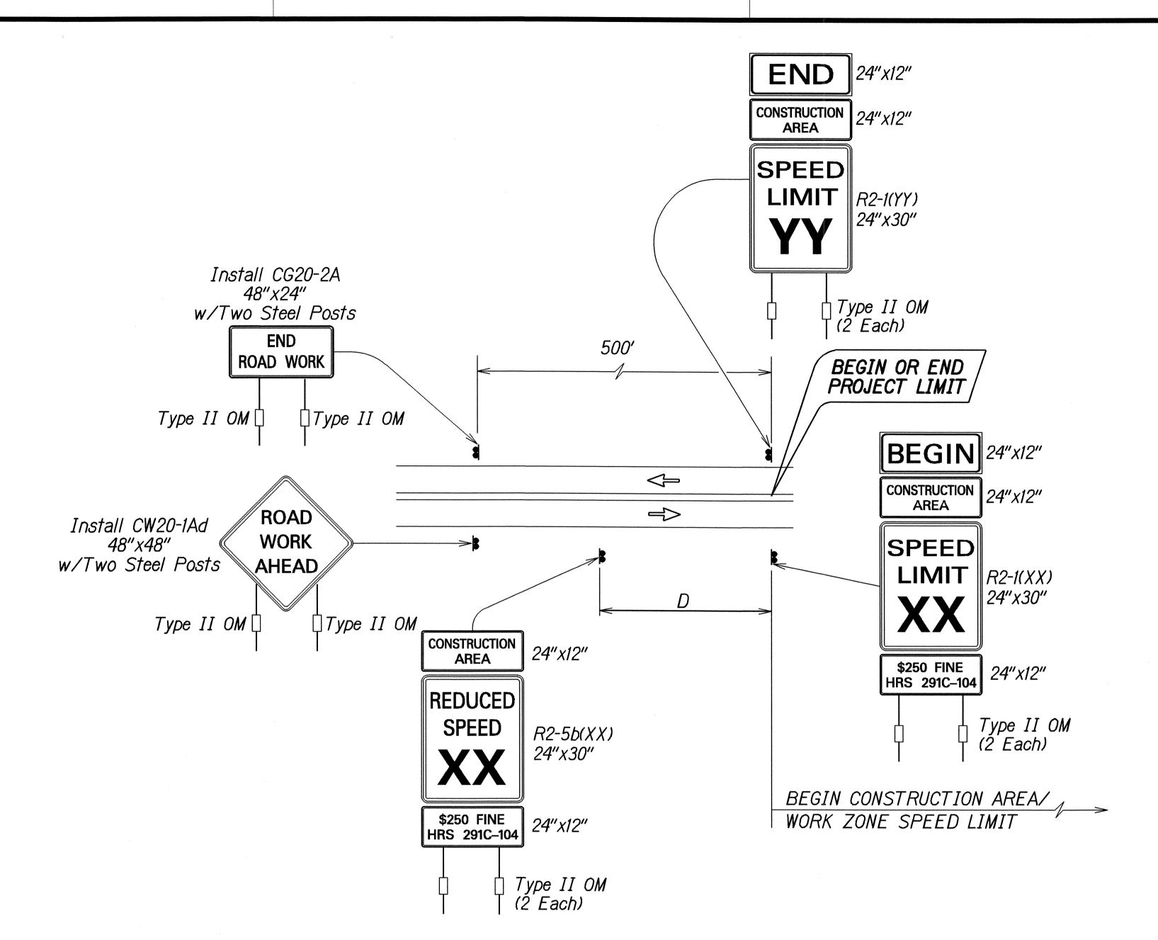
TYPICAL DETAIL FOR CONSTRUCTION SIGNS
