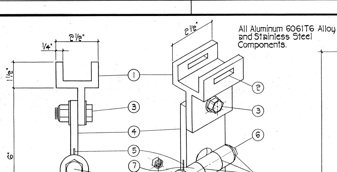
sign mounting hole to bottom of bracket FIXED LENGTH NON-ADJUSTABLE SWING SIGN BRACKET Not to Scale
