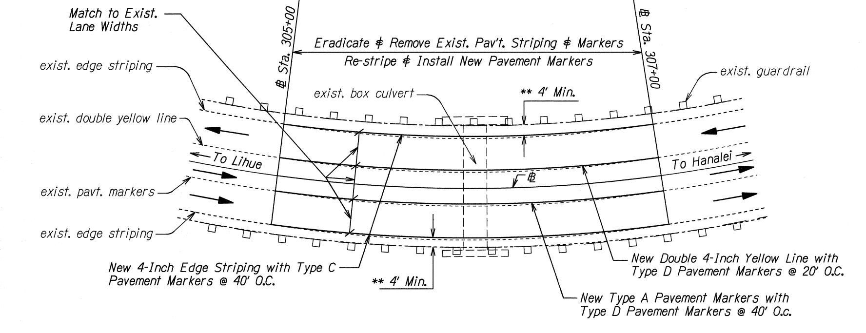
RE-STRIPING PLAN BETWEEN STA. 305+00 AND STA. 307+00
