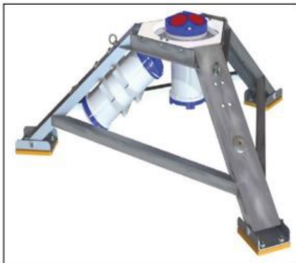
Figure 2. Acoustic Doppler Current Profilers installed on corrosion resistant aluminum Deepwater Buoyancy's BTM-AL50 bottom mounts holding the equipment in place.
