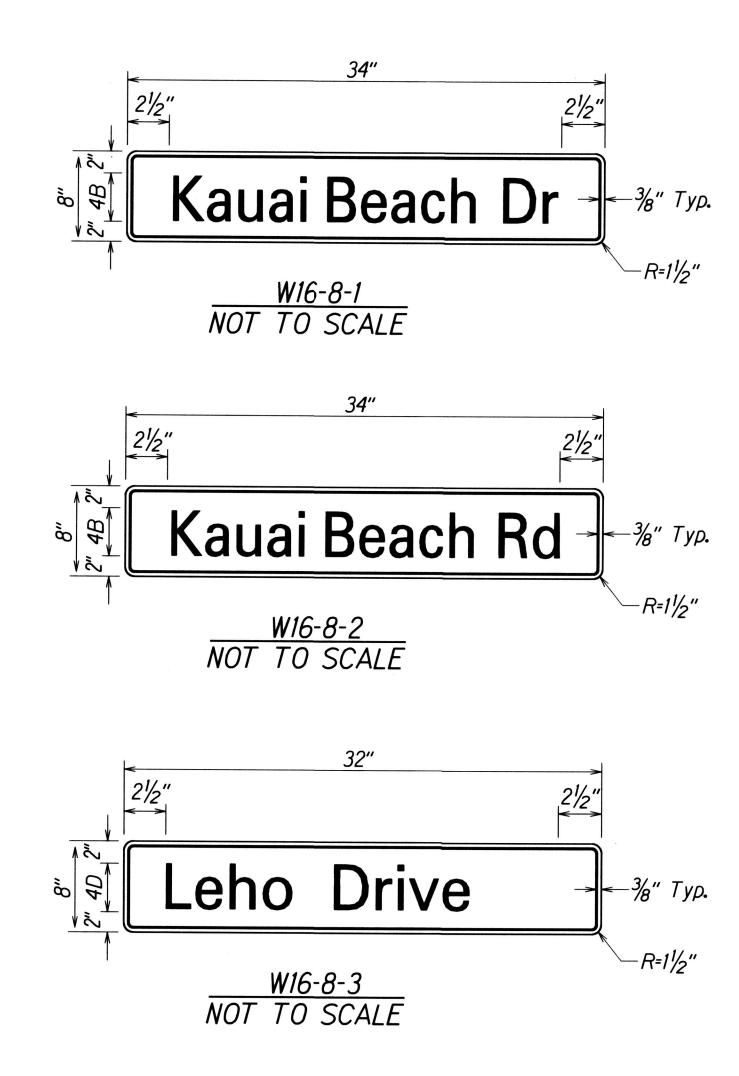
Note: Advance Street Name Sign (W16-8) shall be installed on intersection warning sign (W2-2) and shall have black lettering and borders on a yellow background. Width of borders shall be  $\frac{5}{8}$ ".
