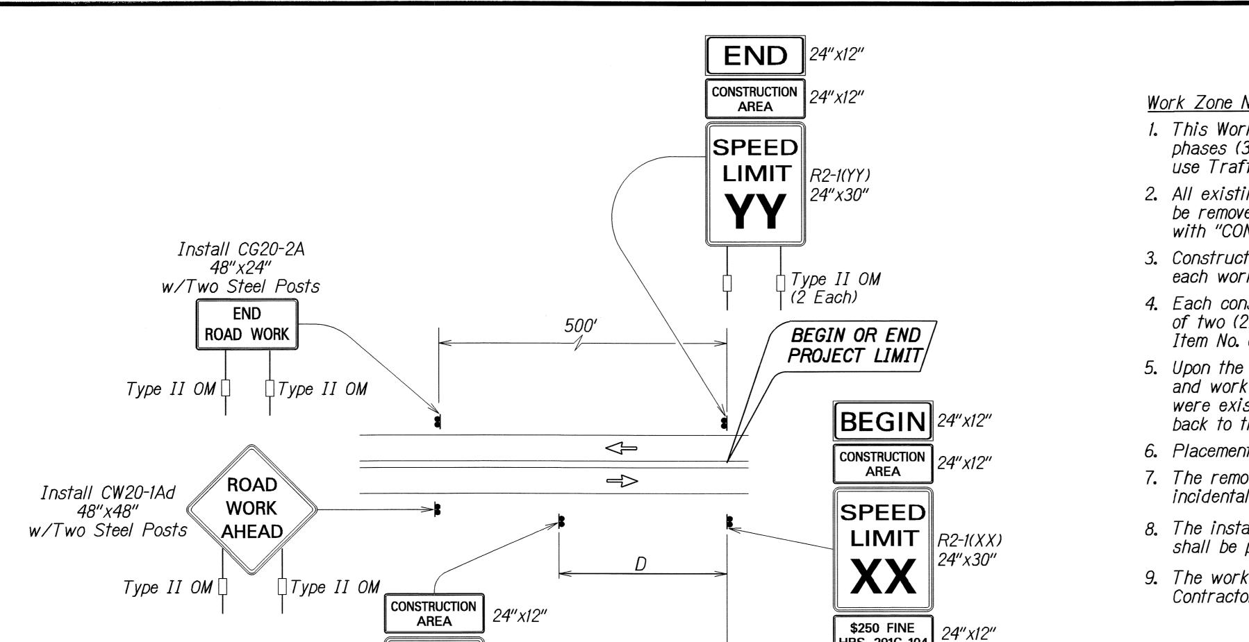
TYPICAL DETAIL FOR CONSTRUCTION SIGNS ON TWO LANE OR MULTILANE UNDIVIDED LOW SPEED HIGHWAY
