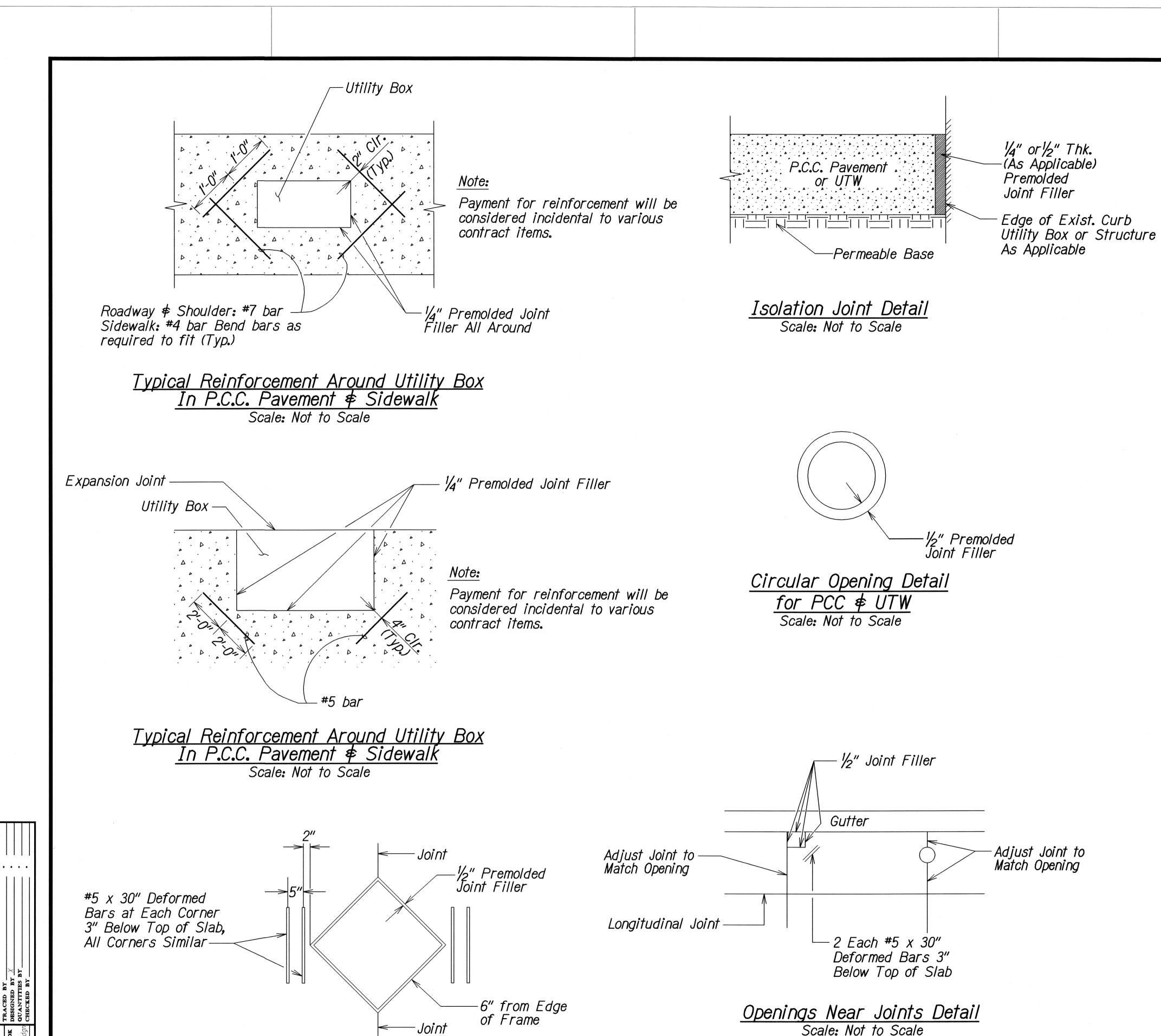
Openings With Corners - Corners At A Joint Detail
