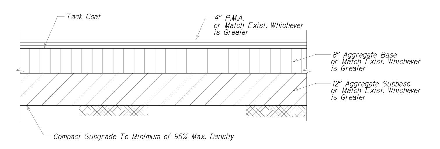
Typical A.C. Pavement Section - Kaumualii Highway/Waimea Canyon Drive Not To Scale
