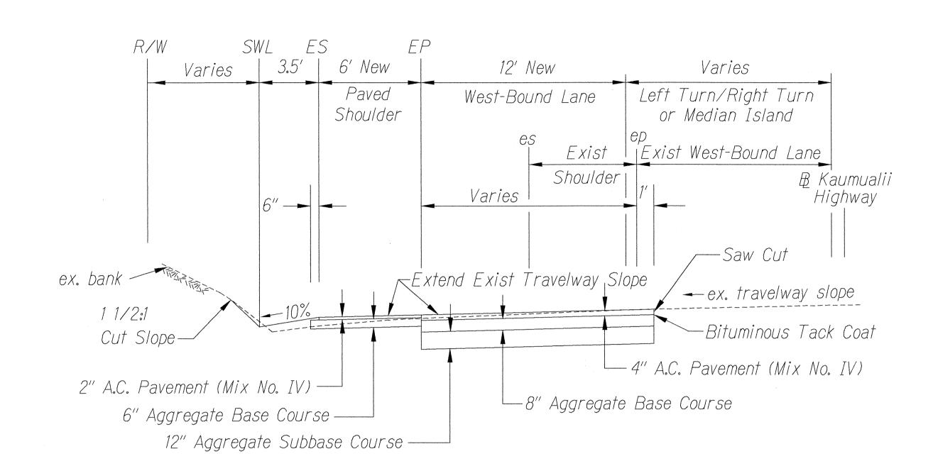
TYPICAL SECTION KAUMUALII HWY. B STA. 194+50 TO B STA. 196+50 Scale: 1" = 4'
