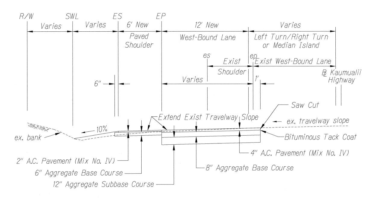
TYPICAL SECTION KAUMUALII HWY. B STA. 192+20.50 TO B STA. 194+00 Scale: 1" = 4"
