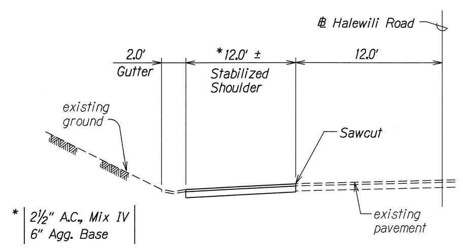
TYPICAL SECTION AT GUTTERS HALEWILI ROAD ₱ STA. 50+78± TO ₱ STA. 57+00 ± 0/S LT. Scale: 1/4"=1'-0"
