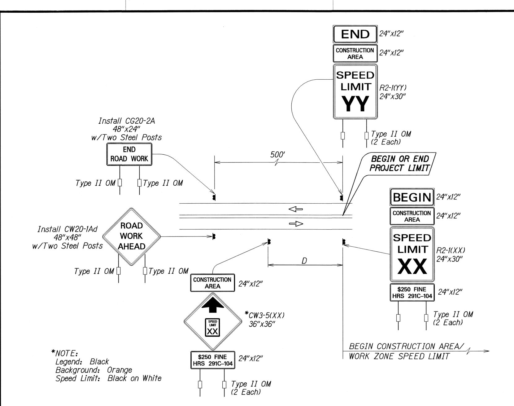
TYPICAL DETAIL FOR CONSTRUCTION SIGNS
