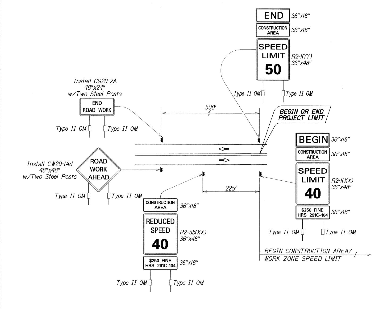
TYPICAL DETAIL FOR CONSTRUCTION SIGNS
