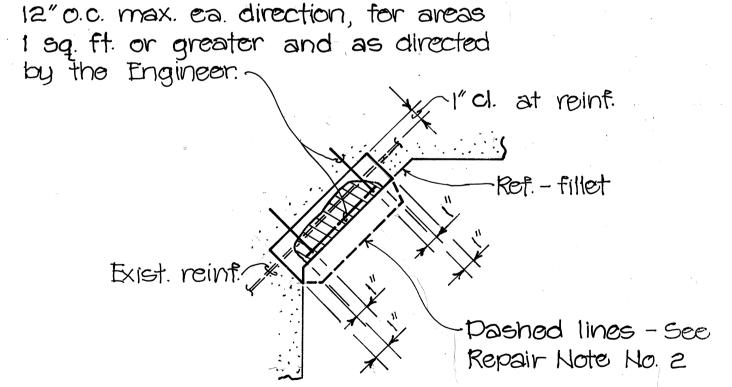
Welded wire fabric, 2×2-W1.4×W1.4
