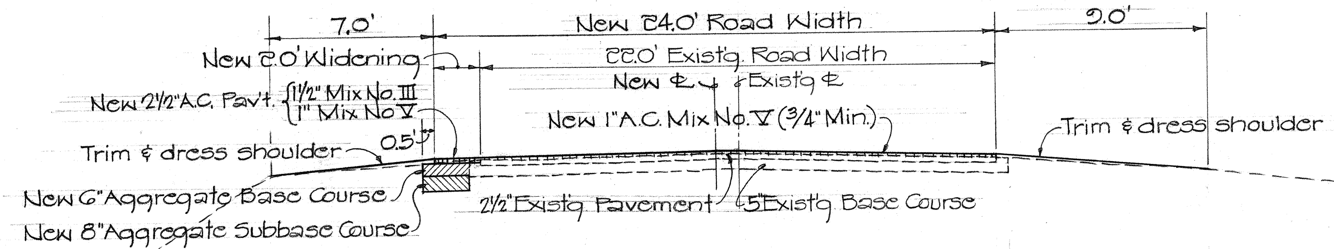
TYPICAL SECTION ON TANGENT 10' WIDENING ON BOTH SIDES & RESURFACING Scale: 1/4" = 1'-0"
