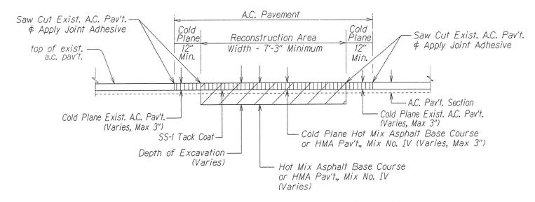
Note: Reconstruct weakened pavement areas prior to cold plane
