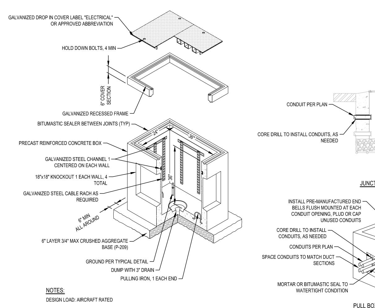
1. UNLESS OTHERWISE SPECIFIED, THE PULL BOX SHALL BE PRE-CAST CONCRETE, AIRCRAFT RATED FOR 100,000LBS LOAD
