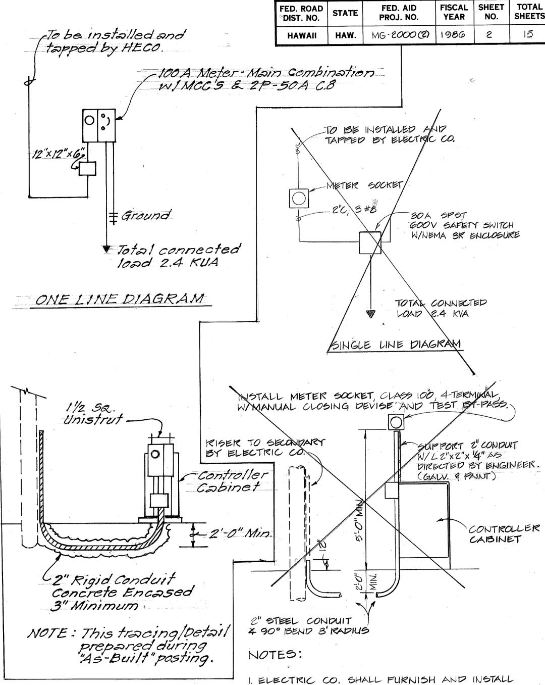
I, ELECTRIC CO. SHALL FURNISH AND INSTALL CABLE BETWEEN SECONDARY AND METER SOCKET.
