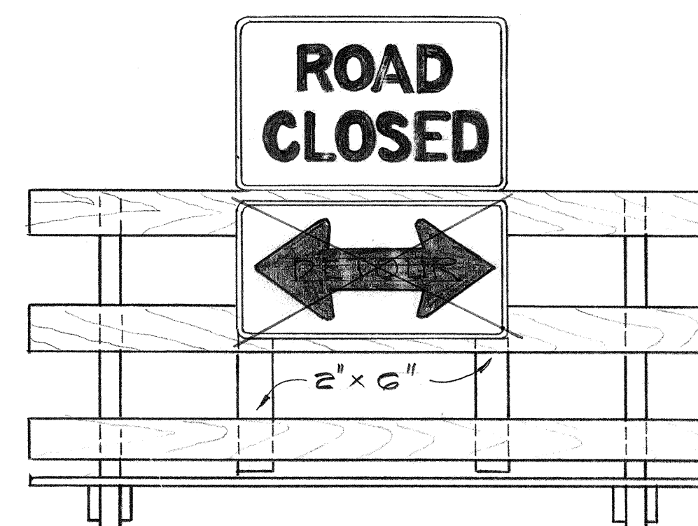
DETAIL OF WOOD BARRICADE (TYPE III)
