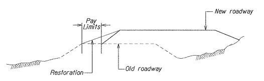
Restoration in this and similar cases will not be measured for payment under item 21101 if the slope stake is modified to encompass the restored area.
