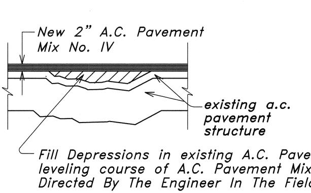
Fill Depressions in existing A.C. Pavement With leveling course of A.C. Pavement Mix No. V, As Directed By The Engineer In The Field.
