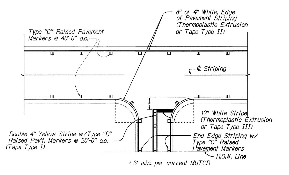
TYPICAL EDGE OF PAVEMENT MARKING
