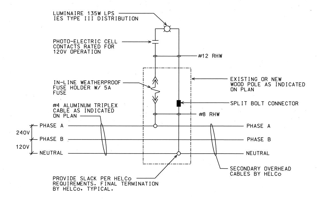
A TYPICAL STREET LIGHT WIRING DIAGRAM
