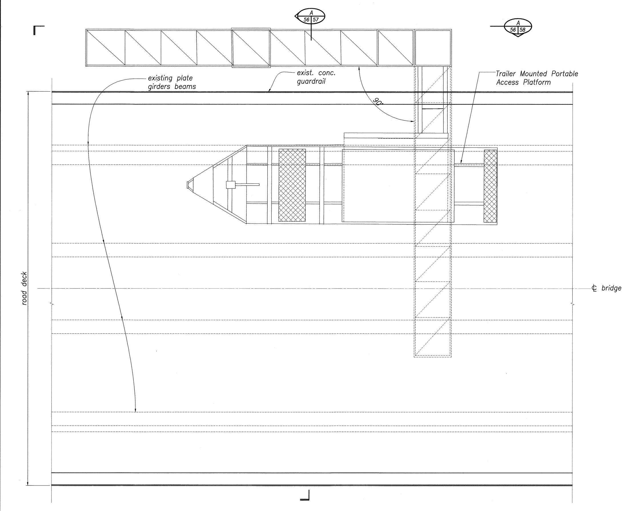
PORTABLE ACCESS PLATFORM SYSTEM PLAN
