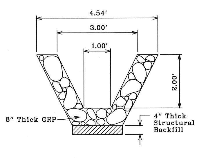
DITCH SECTION - STATION 0+22.2 TO 0+26.87 Not To Scale
