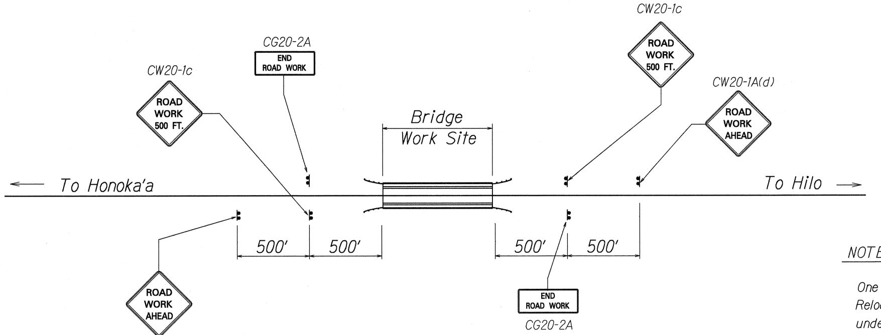
CONSTRUCTION SIGN PLAN FOR NON-WORKING HOURS Not To Scale
