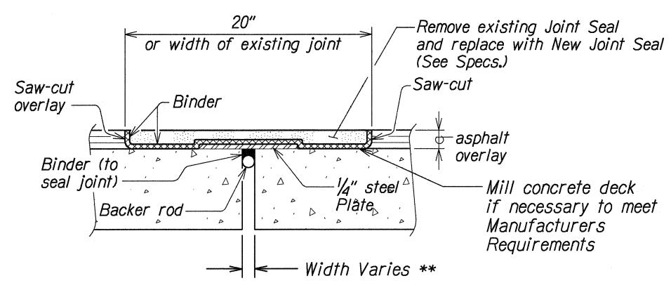
\*\* NOTE: Contractor shall verify width in the field prior to pre-fabricating and ordering of materials. Contractor to fabricate and install per Manufacturers specifications.
