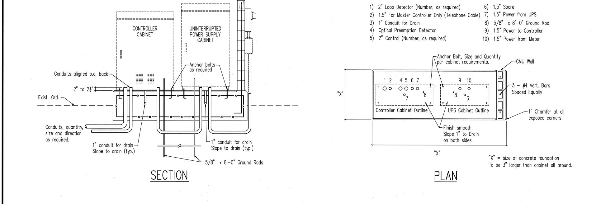
CONTROLLER, UPS, & METER PEDESTAL FOUNDATION
