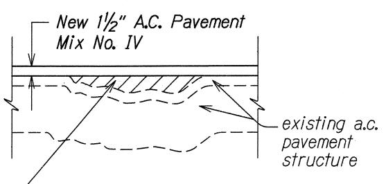
Fill Depressions in existing A.C. Pavement With leveling course of A.C. Pavement Mix No. V, As Directed By The Engineer In The Field.
