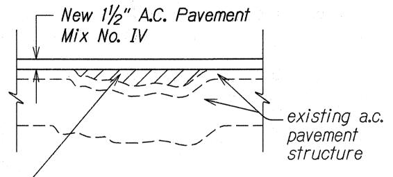
Fill Depressions in existing A.C. Pavement With leveling course of A.C. Pavement Mix No. V, As Directed By The Engineer In The Field.
