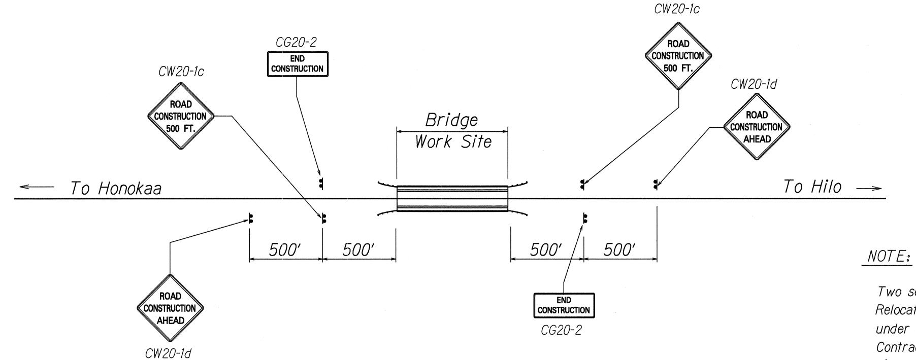
CONSTRUCTION SIGN PLAN FOR NON-WORKING HOURS
