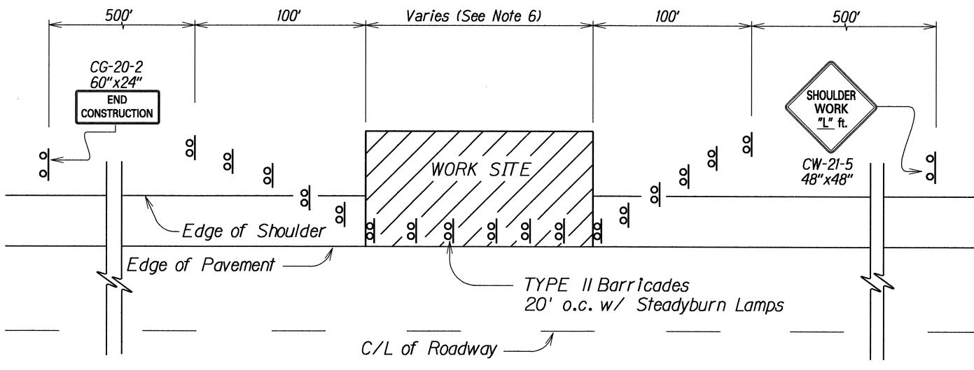
TRAFFIC CONTROL PLAN FOR USE DURING NON-WORKING HOURS
