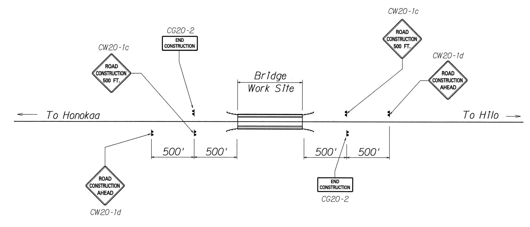
CONSTRUCTION SIGN PLAN FOR NON-WORKING HOURS
