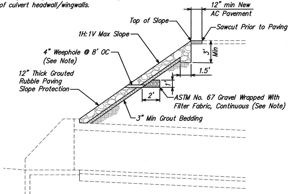
GROUTED RUBBLE PAVING SLOPE PROTECTION
