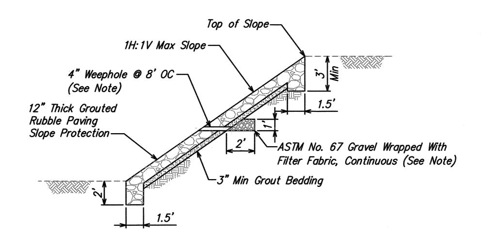
(4) GROUTED RUBBLE PAVING SLOPE PROTECTION
