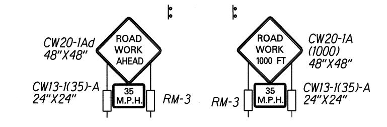
TYPICAL DIAGRAM FOR CONSTRUCTION SIGN LAYOUT
