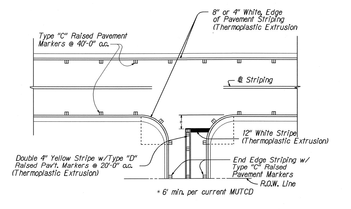
TYPICAL EDGE OF PAVEMENT MARKING
