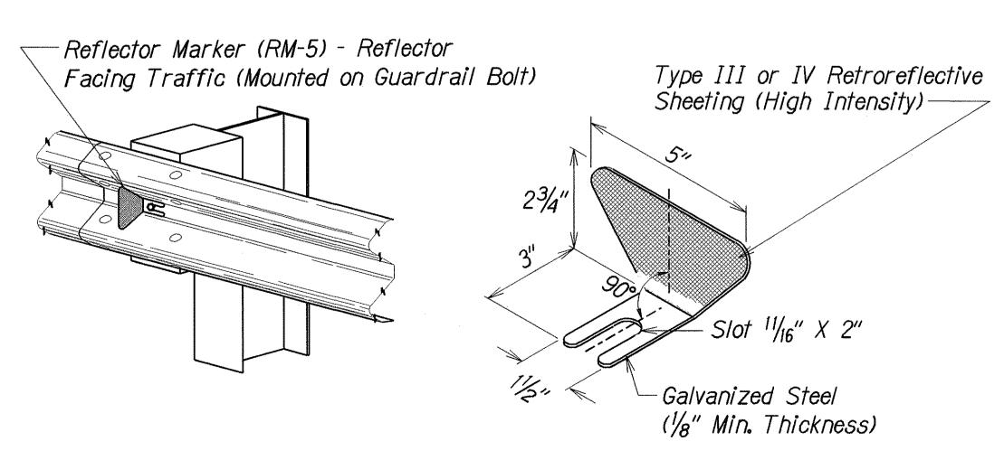
REFLECTOR MARKER (RM-5) DETAIL AND TYPICAL INSTALLATION
