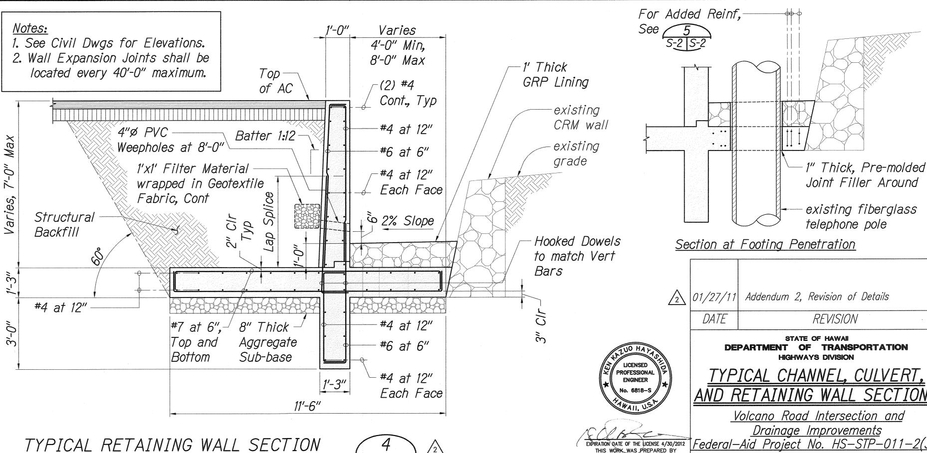
TYPICAL CHANNEL, CULVERT, AND RETAINING WALL SECTIONS Volcano Road Intersection and
