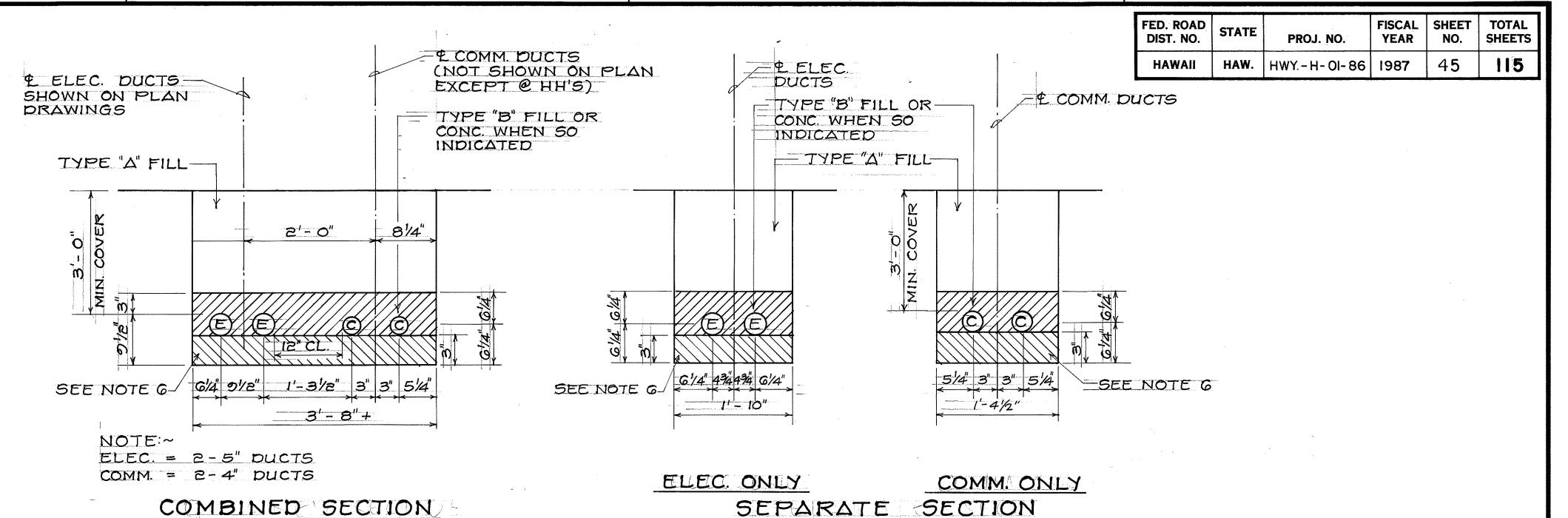
TYPICAL DIRECT BURIED DUCT SECTIONS
